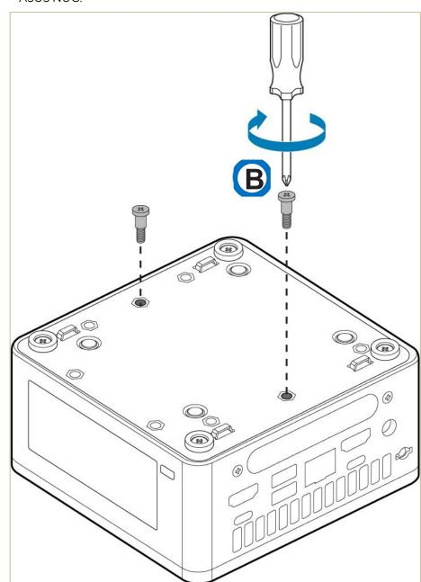
2. Attach the two slightly larger black screws to the bottom chassis cover of the ASUS NUC.
