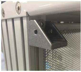
After the panel is removed, add the triangle bracket to the left or right metal extrusion upright (as shown in Figure 2) using the M5 x 22 mm Cap Head Screw (MGSUBS1A) and M4 Allen Wrench. Left mounted triangle bracket is for a right offset tray, and right mounted triable bracket is for a left offset tray.
